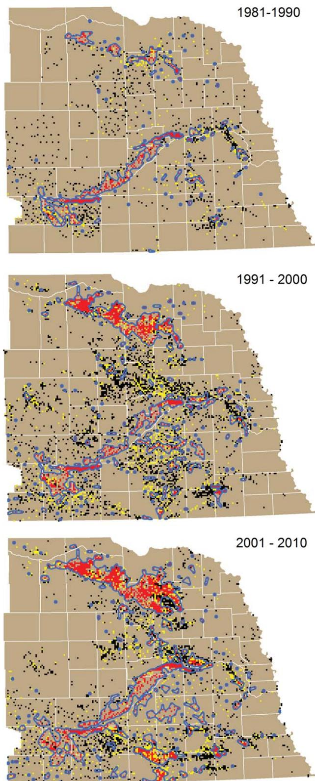
**Figure 2.** Decadal emergence of contaminated ( $\geq 10$  mg N/L) groundwater. In each decade, the highest nitrate concentrations in irrigation wells within 2 km by 2 km grid cells were averaged. Black cells depict average concentrations  $< 5$  mg N/L, yellow cells 5 to  $< 10$  mg N/L, and red cells  $\geq 10$  mg N/L. The red grid cells were the basis for modeling the  $\geq 10$  mg N/L contaminated areas outlined in blue.
