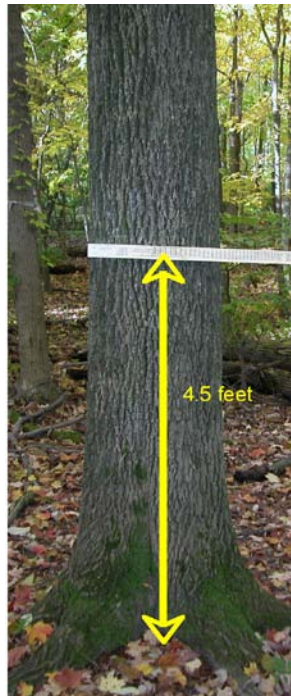
Figure 2a. The stick should be placed against the tree 4½ feet from the ground.
