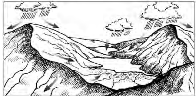
Fig. 1-4. A watershed is the area defined by upland ridges that direct waters to a specific waterbody.
