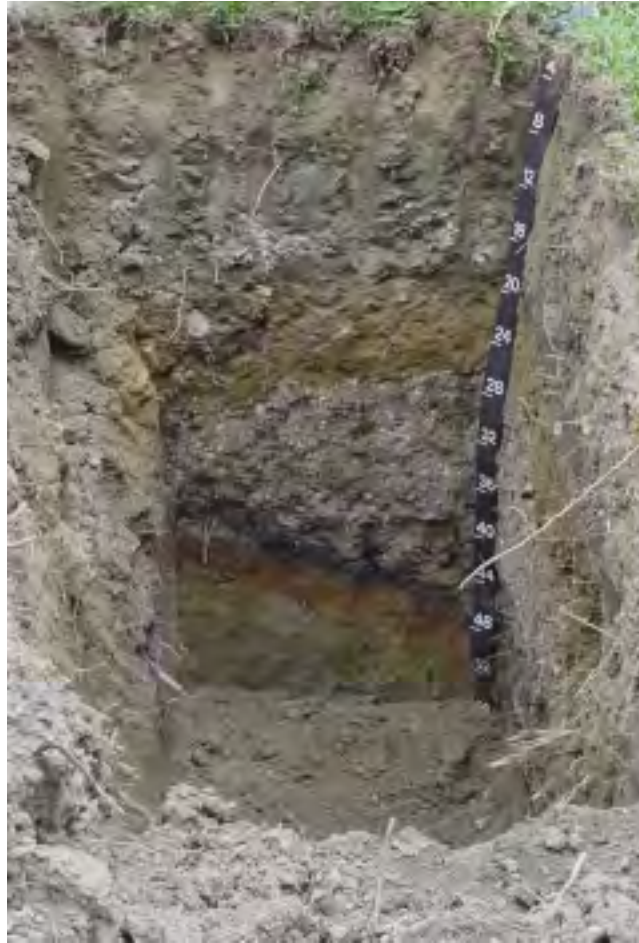
Figure 4.8: Soil profile with a buried layer of ash and refuse. This site was burned by a city fire.
