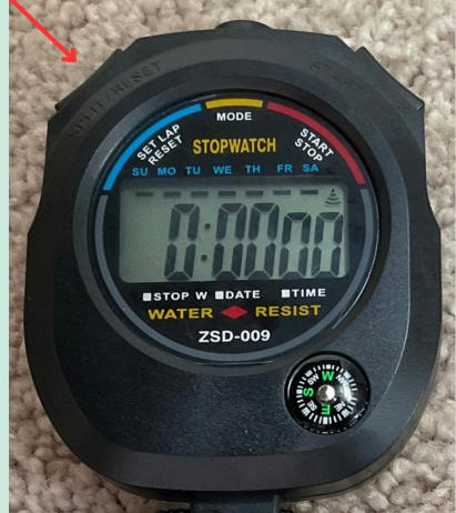
To reset the timer back to zero, press the RESET button only after stopping the time
