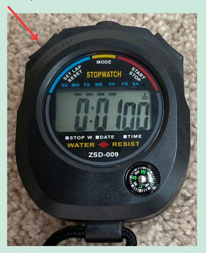
When you reach the stopwatch screen, it will typically start at all zeros. If it does not, press the RESET button to clear any previously recorded time.
