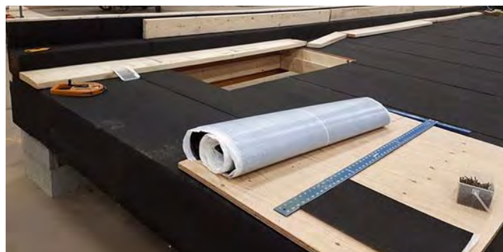
The building of a road infrastructure physical model, using wood and tar paper.
