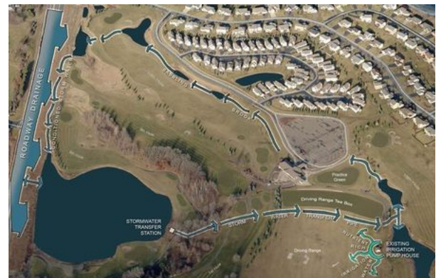
Plan for the harvest system showing storage and transport components. Image courtesy Emmons and Olivier Resources, HR Green and Water in Motion.
