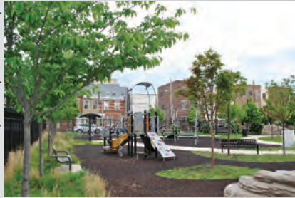
A porous play surface made from recycled tires is surrounded by rain gardens and trees.
