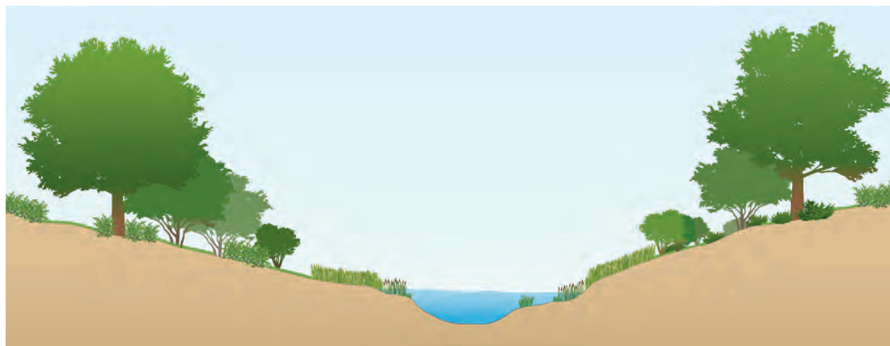
Figure 2-9. Along a stream, a vegetated riparian buffer protects the channel, filtering sediment, nutrients, and other pollutants.
