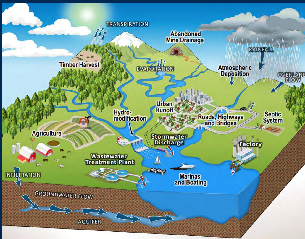
Figure 1: Examples of Point and Nonpoint sources of Pollution in a Watershed. Credit EPA
